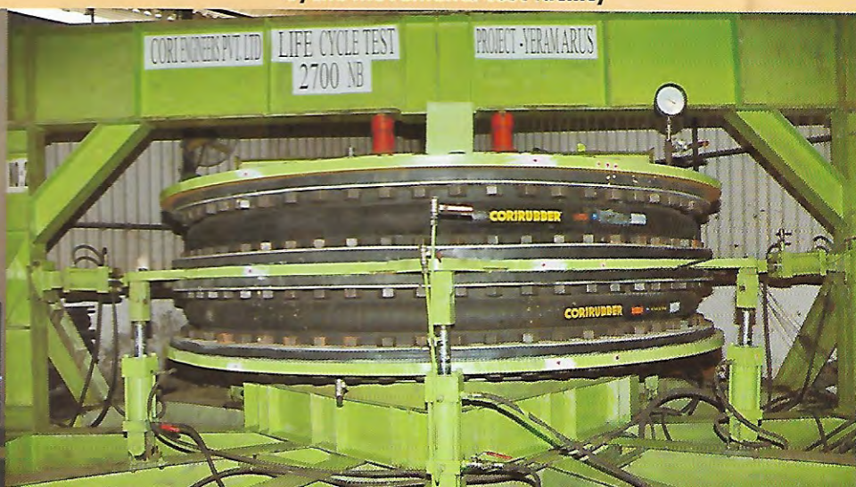
Cyclic movements test facility
